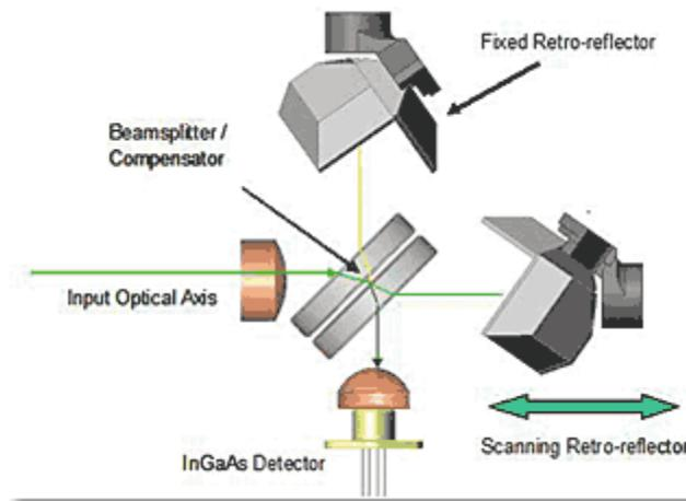
**Figure 1.** Our Fourier transform spectrometer (FTS) is based on a Michelson configuration. Moving the scanning retro-reflector phase shifts the two beam paths relative to each other, producing sinusoidal intensity variations at the detector that have frequencies proportional to the wavelengths of incoming light.
