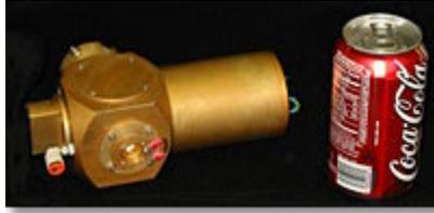
*Custom, compact FTIR makes noninvasive alcohol measurements commercially viable.*
